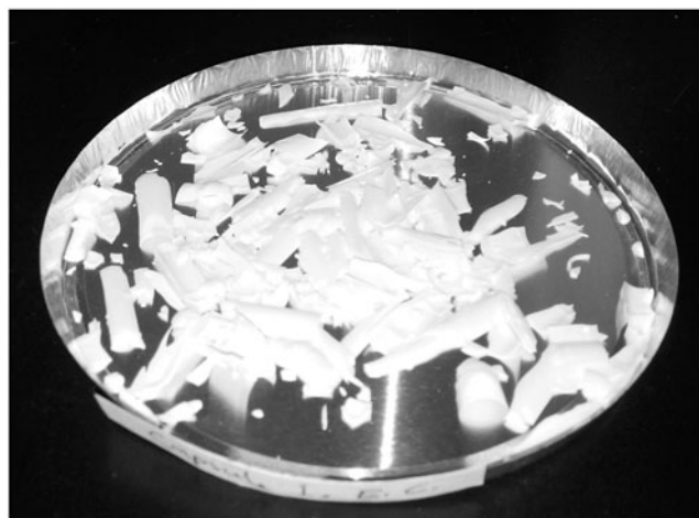
Figure 3. Fragments of dried Capsule 1 following the free fall of 300 g weight over 30 cm height.
